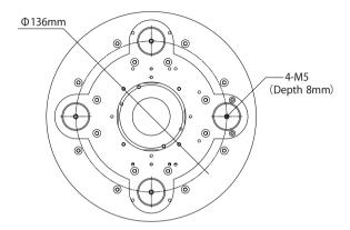
Figure: Fixing screws
