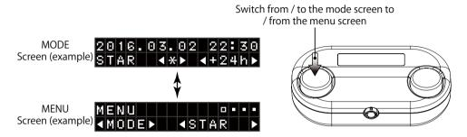
Figure: Switch from / to the mode screen to / from the menu screen
