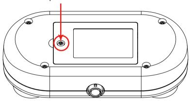
Figure: Removing the battery cover
