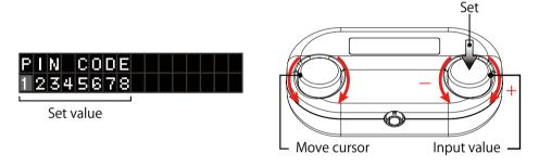
Figure: Setting pin code
