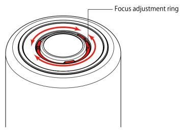
Figure: How to focus the projection lens
