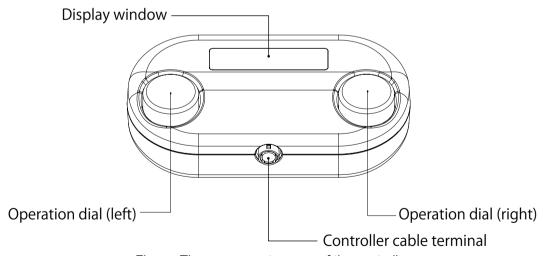
Figure: The component names of the controller
