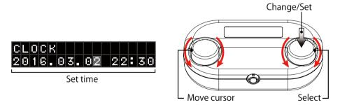
Figure: Setting internal clock
