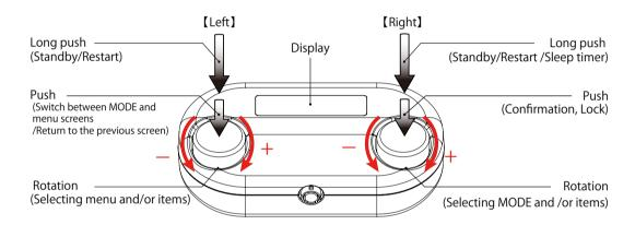
Figure: How to operate the controller
