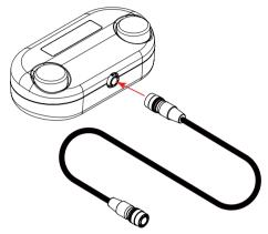
Figure: Connect the controller with its cable
