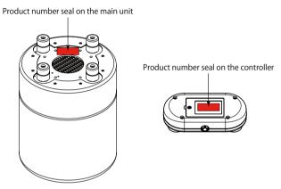
Figure: Check the serial number
