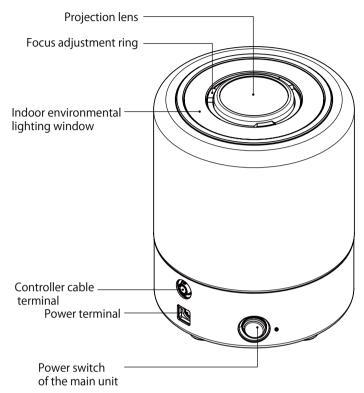
Figure: The component names of the main unit
