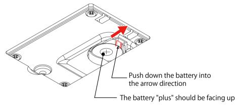
Figure: Removing the battery
